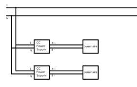
DO NOT interconnect wires with different colors. Please consider the TOTAL ADDRESSES before wiring.
